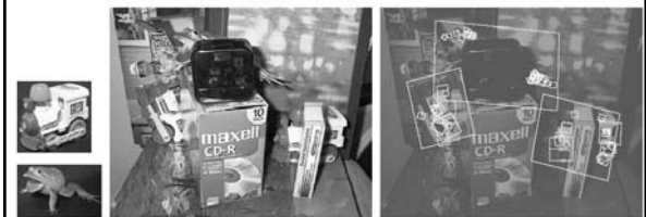
Figure 12: The training images for two objects are shown on the left. These can be recognized in a cluttered image with extensive occlusion, shown in the middle. The results of recognition are shown on the right. A parallelogram is drawn around each recognized object showing the boundaries of the original training image under the affine transformation solved for during recognition. Smaller squares indicate the keypoints that were used for recognition.
