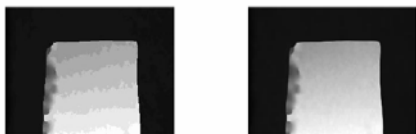
Figure 7. Comparison of MAP and MMSE estimates on a different MRF formulation. The MAP estimate chooses the most likely discrete disparity level for each point, resulting in a depth-map with stair-stepping effects. Using the MMSE estimate assigns sub-pixel disparities, resulting in a smooth depth map.
