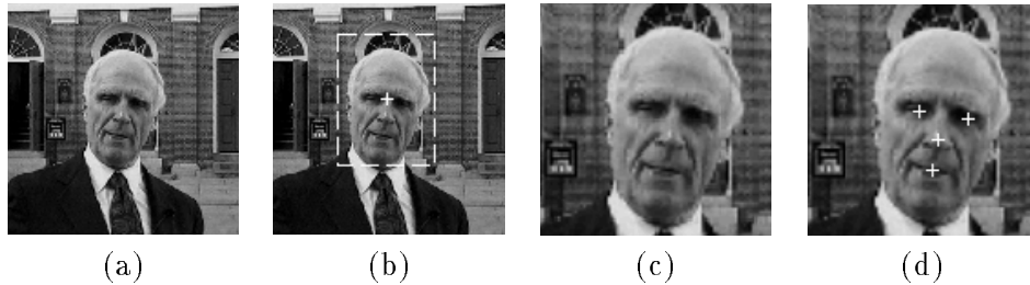
Figure 8: (a) original image , (b) position and scale estimate , (c) normalized head image , (d) position of facial features .
