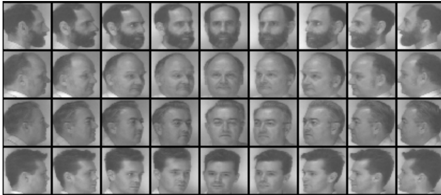
Figure 12: Some of the images used to test accuracy at face recognition despite wide variations in head orientation. Average recognition accuracy was 92%, the orientation error had a standard deviation of 15^\circ .
