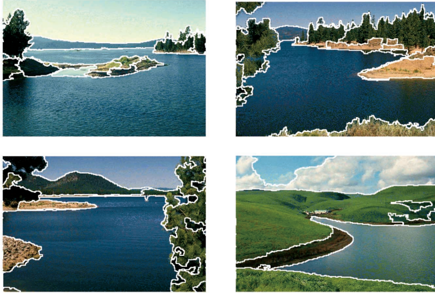
Fig. 10. Landscape images. All the region boundaries were delineated with (h_s, h_r, M) = (8, 7, 100) and are drawn over the original image.
